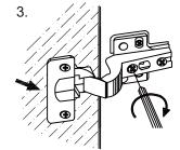
MOVE DOOR OUTWARD by turning this screw clockwise
