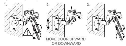
Unscrew 2 screws in round holes loosen 2 screws in oval holes a bit.
